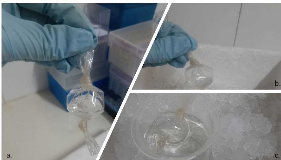
Figure 1. Dialysis Stages: a. Transfer of the protein solution into the membrane and removal of the air inside, followed by tying the other end. b. Dialysis membrane with the protein solution inside, removing the air, and tying the other end. c. Immersion of the dialysis membrane into at least 10 times its volume of dialysis buffer (pure water).
